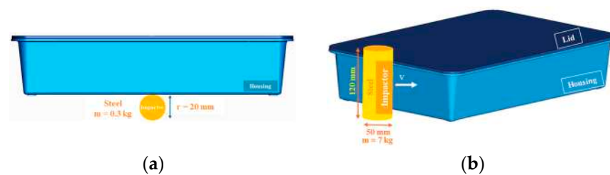
Figure 2. Impactor geometry for (a) ground and (b) pole impact.
